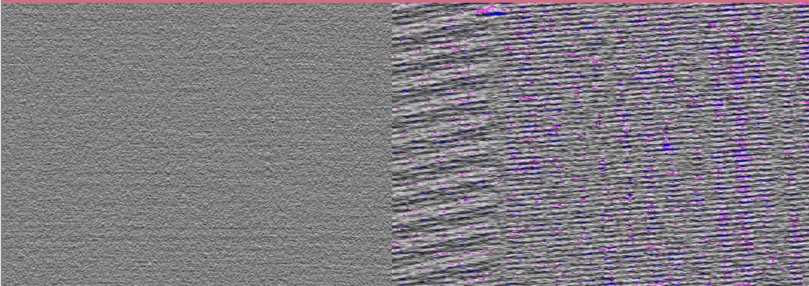
The left figure shows a roll without significant chatter marks. The right figure shows short wavelength chatter marks. In the left area there is a long wavelength chatter frequency below the short wavelength chatter mark.
