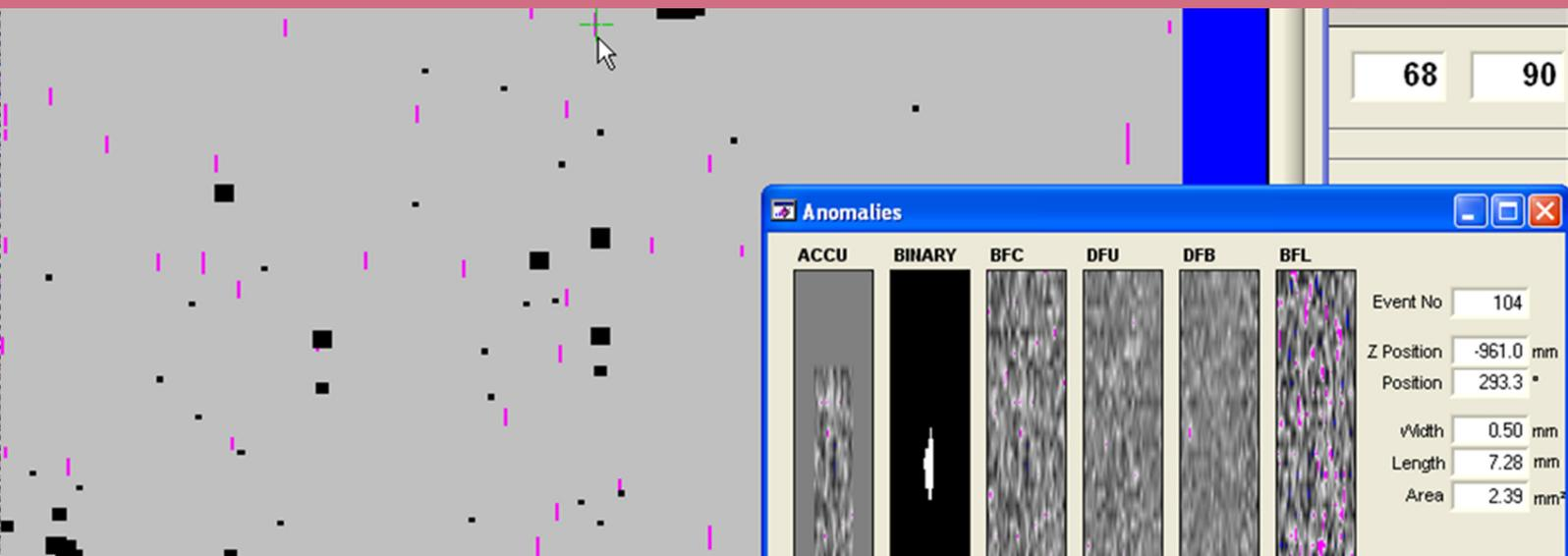
Different classes of Single Defects will be detected and classified through a flexible set of filters.
